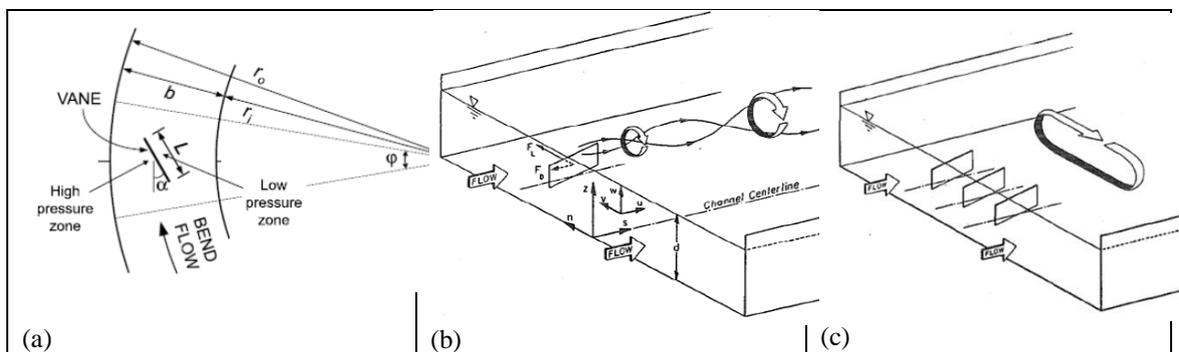
**Figure 1:** (a) Typical vane orientation and location of high and low pressure zones (Voisin and Townsend, 2002) (b) Schematic of flow situation showing vane-induced circulation (Odgaard and Wang, 1991) (c) Schematic showing circulation induced by array of three submerged vanes (Odgaard and Wang, 1991).
