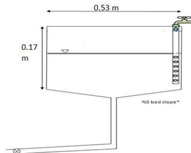
Figure 3: Typical scheme of laboratory 'Cornell-type' dual-drain tank.
