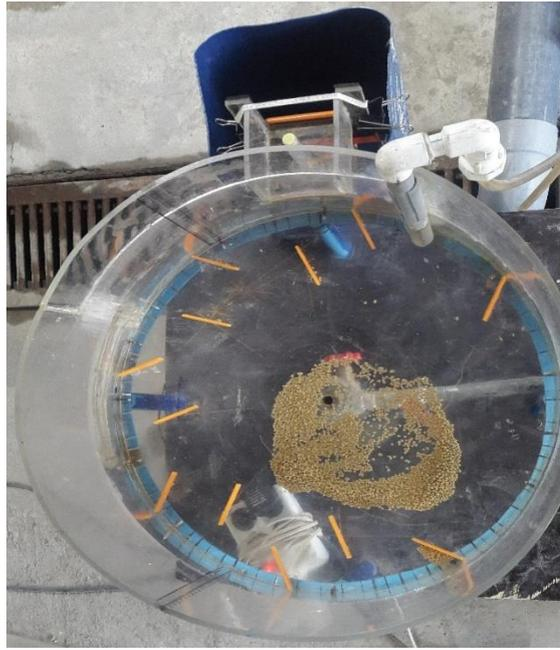
**Figure 4: Sample of sedimentation in cylindrical tank.**
