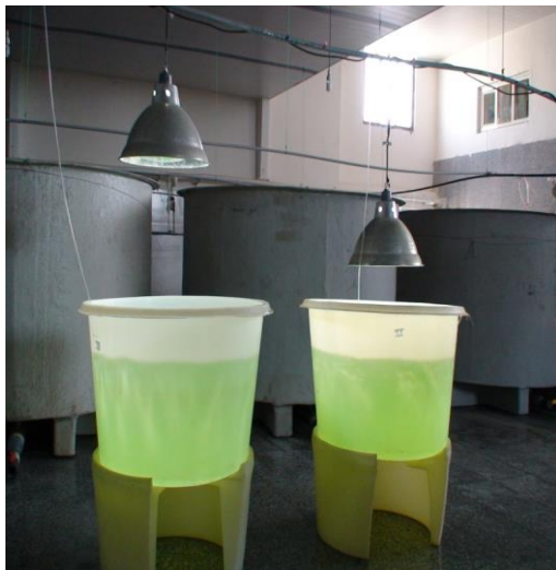
Figure 1: Adjusting of light intensity by changing the distance of light source from the water surface.
