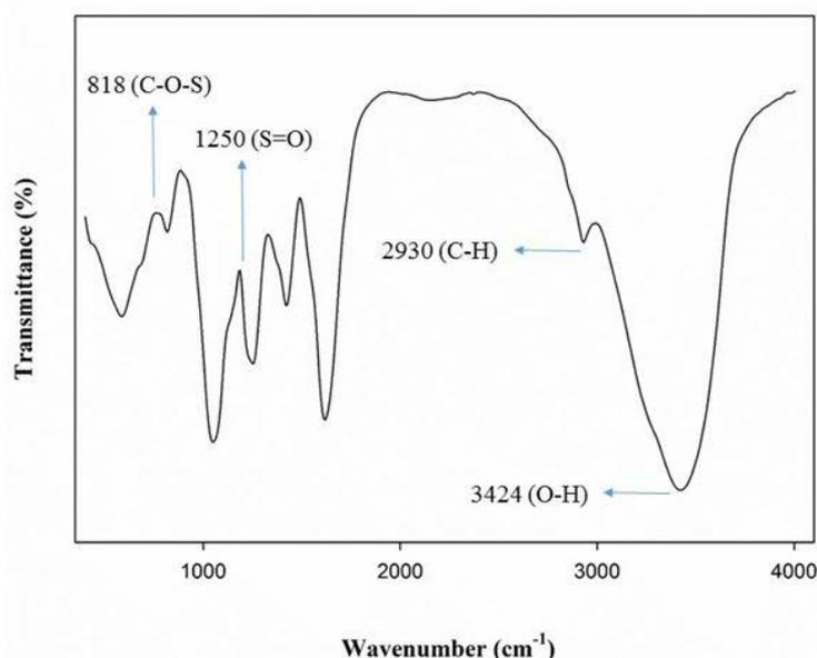
**Figure 1:** FT-IR spectra of fucoidan extracted by ultrasonic/microwave (UM) method.
